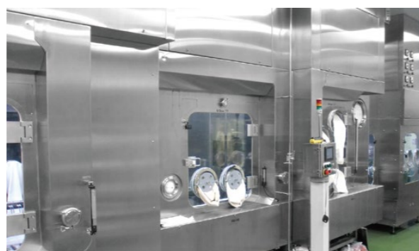
Vial filling line Sterilization + Containment
